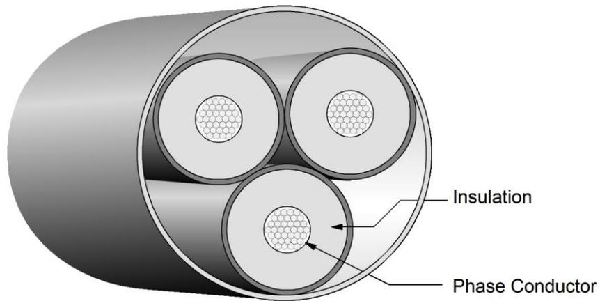
**Figure 3.23: Three-Phase Medium Voltage Cable**
