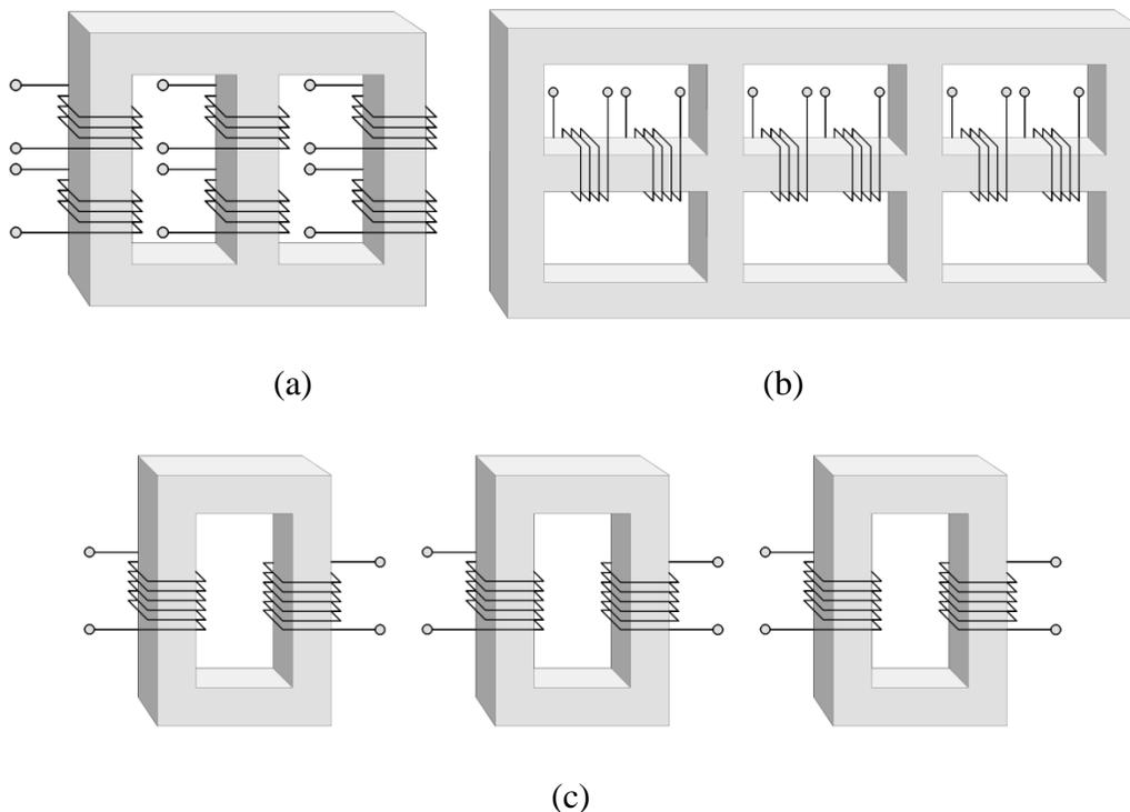
**Figure 3.27: Three Phase Transformers**
