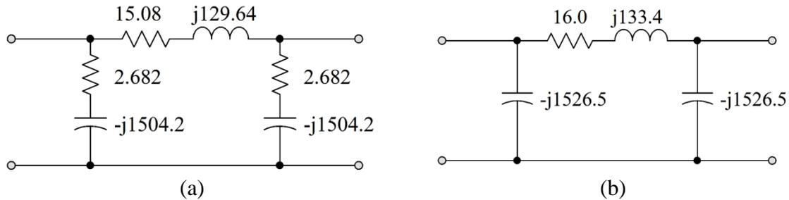
**Figure E3.6: The Positive Sequence Equivalent Circuits**
