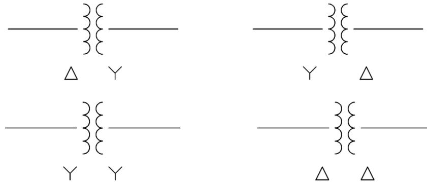
**Figure 3.28: Schematic Representation of Three Phase Transformers**
