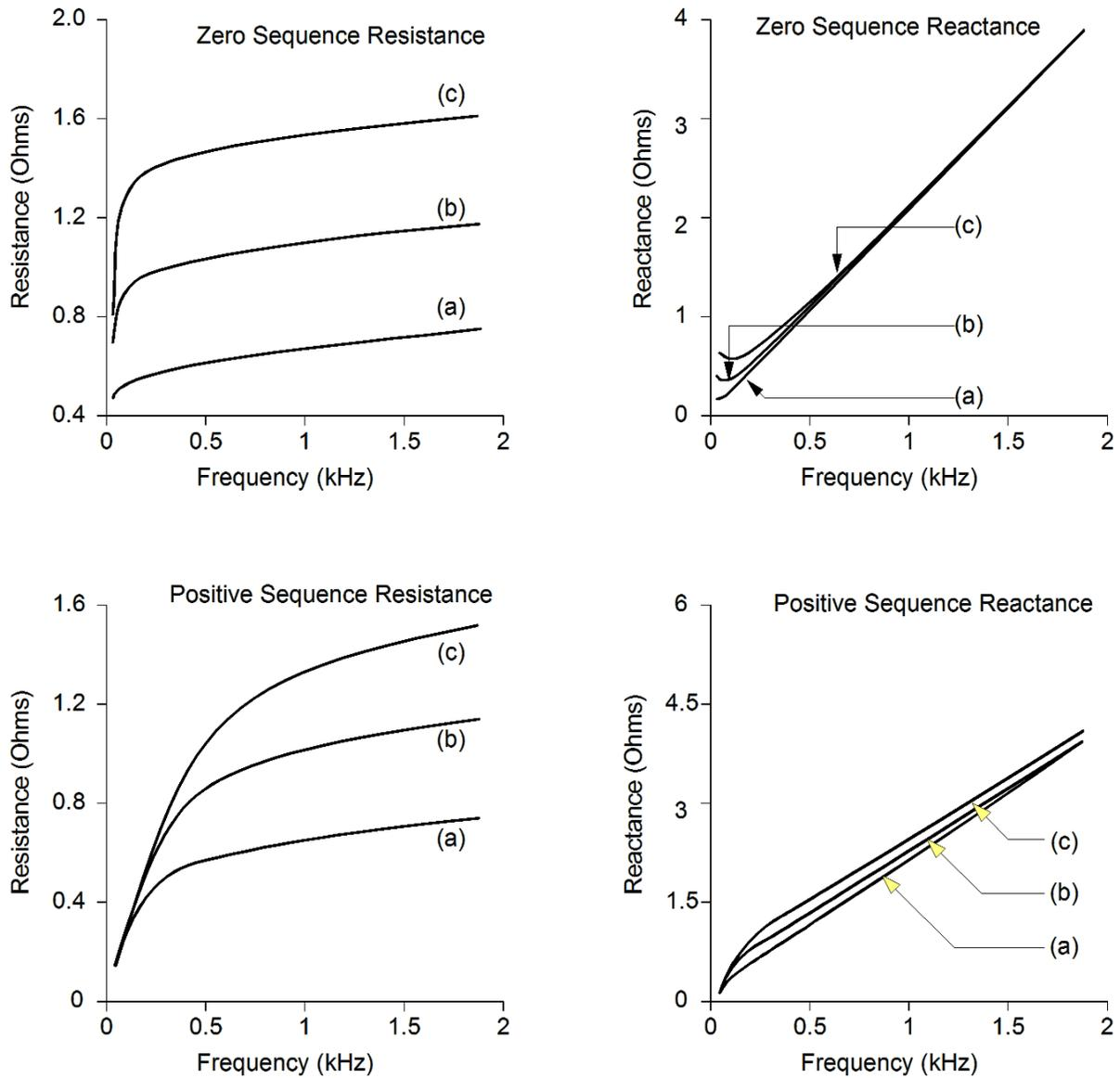
**Figure 3.25: Parametric Analysis of 15 kV Concentric Neutral Cable Sequence Parameters**
