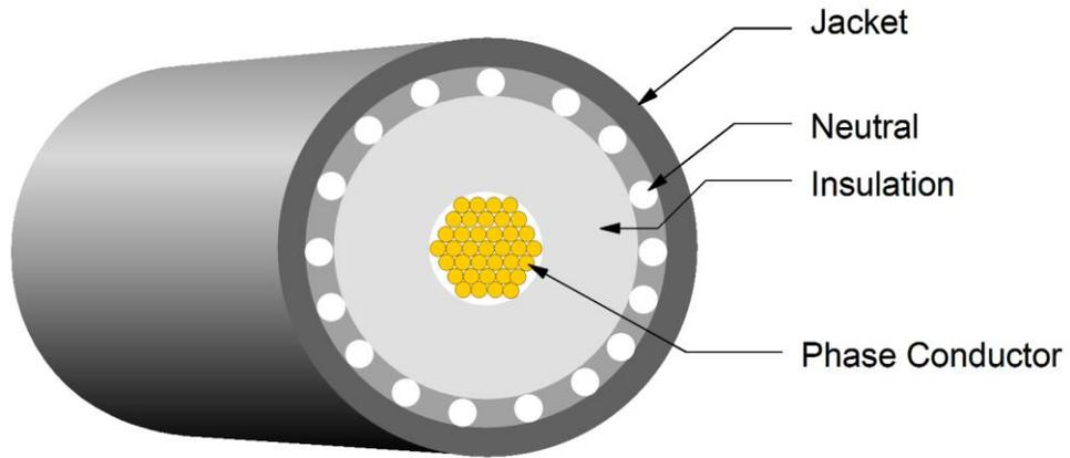
**Figure 3.22: Concentric Neutral Medium Voltage Cable**
