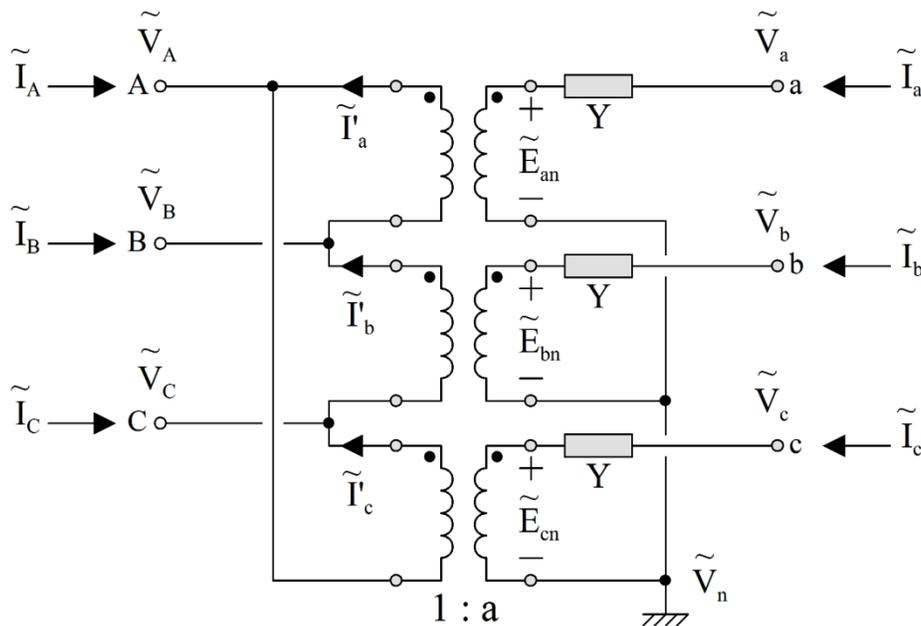
**Figure 3.29: Delta-Wye Connected Three Phase Transformer Model**
