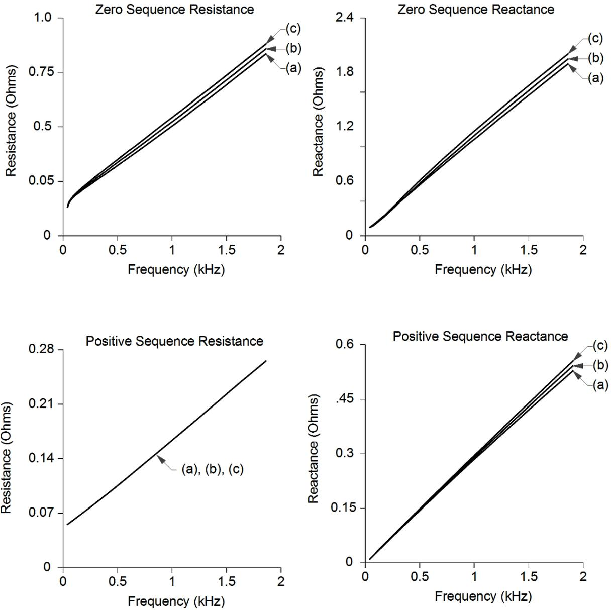
**Figure 3.26: Parametric Analysis of 600 V Cable Sequence Parameters**
