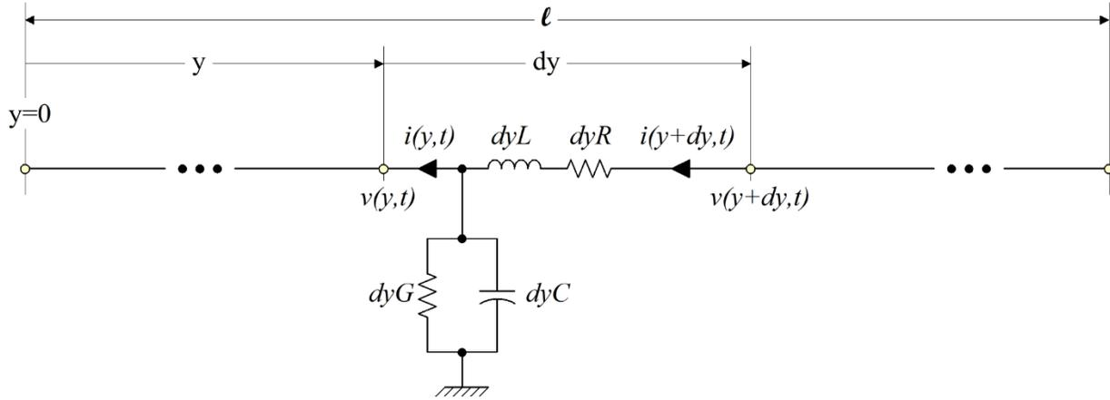
**Figure 3.20: Transmission Line with Distributed Parameters**
