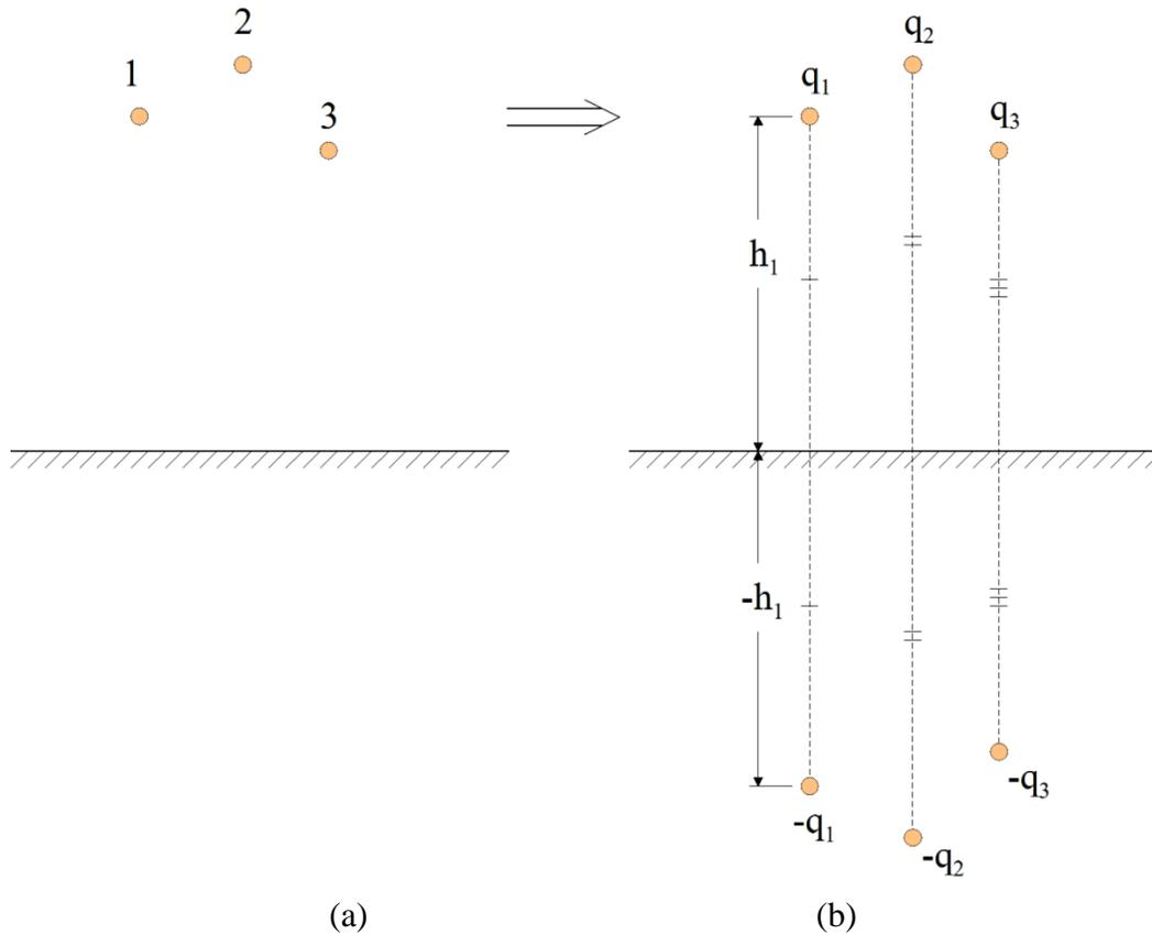
**Figure 3.19: Multi-conductor Line Above Earth**
