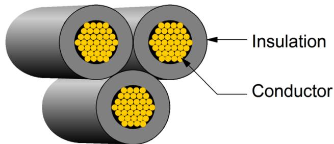
**Figure 3.24: Secondary System 600V Class Cable**
